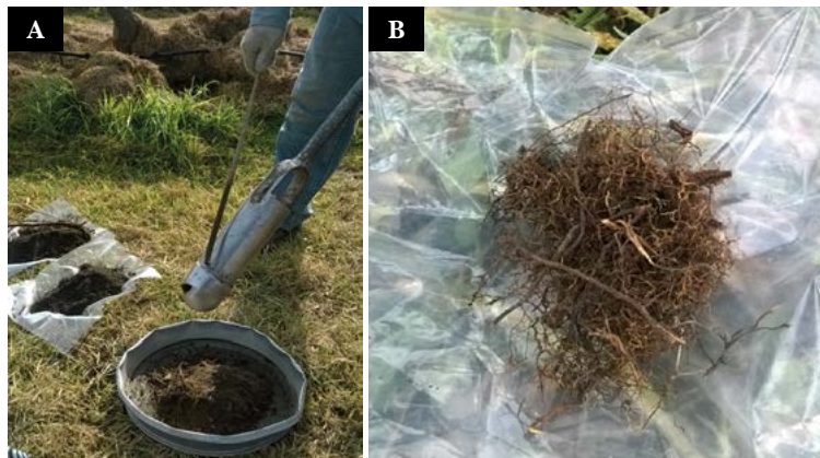
Figure 3. A) Sampling of the roots was made with a California Sampler; B) 330 cm 3 root sample extracted from a specific depth, at 40 cm away from the trunk following the cardinal points.
