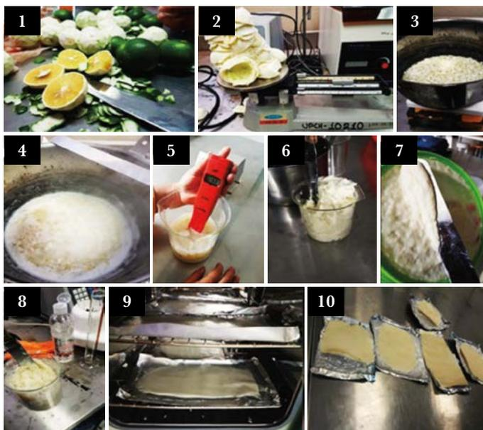
**Figure 1.** Extraction of Bioplastic from orange peel waste (*C. sinensis*). 1) Orange peels; 2) Weighing of shells (mesocarp); 3-4) Hydrolysis; 5) pH measurement; 6) Pectin mass obtained; 7) Pectin sieving; 8) Mixture of pectin with glycerol; 9) Drying of biofilms in a conventional oven; 10) Orange biofilms obtained.
