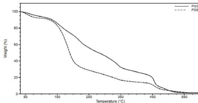
**Figure 5.** TGA curve of orange peel biplastic films.
