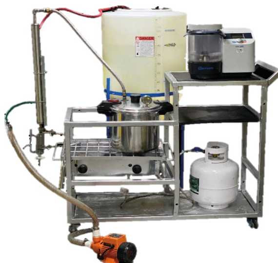
Figure 1. Pilot-scale hydrodistillation apparatus by Armenta et al. , 2023.
