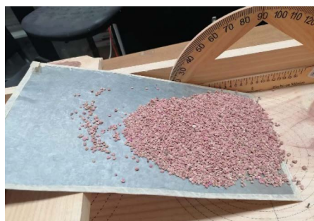
Figure 2. Method for determining the angle of external friction \tan \alpha = \mu_e
