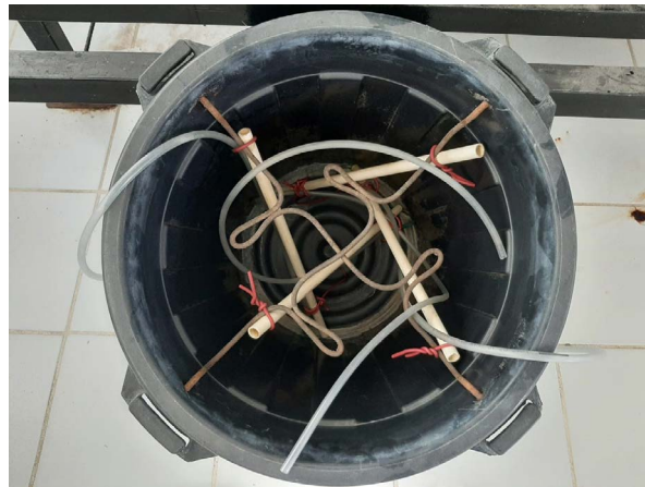
Figure 1. Arrangement of the artisanal Airlift bioreactor.
