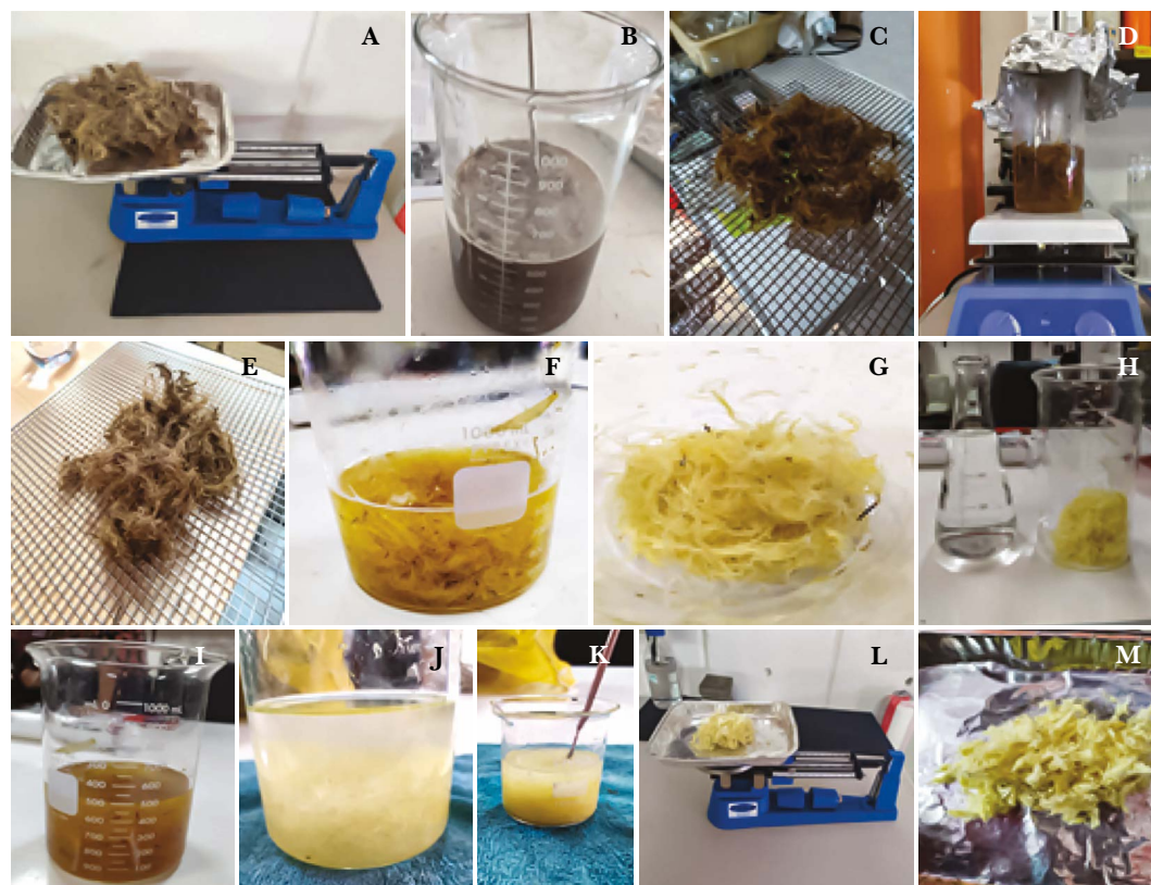
Figure 2. Cellulose extraction process from oil palm bagasse. A: Bagasse weighing; B: Pre-treatment; C: Drying in conventional furnace; D: Acid hydrolysis; E: Drying; F: Chlorination; G: Drying; H-I: Alkaline extraction; J: Blanching; K: Rest; L: Dry fiber/weighing; M: Cellulose.
