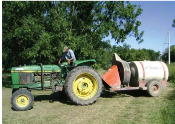
Figure 1. Cannon-type sprayer for the dispersion of entomopathogens.
