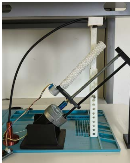
Figure 5. The webcam is equipped with the fitted prototype, which includes the bearing with its base, the blue rigid coupling, and the both structures of the camera, for which the vertical base was designed for positional and height adjustment to ensure the greenhouse tower is captured correctly.
