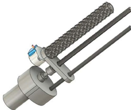
Figure 3. Prototype design and simulation created in Fusion 360, showing the structural components (DC motor, stepper motor, lead screw, rigid coupling, and guide rod).
