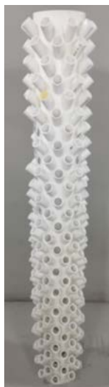
Figure 1. Full-sized greenhouse tower made of PVC material. The tower measures 1.5 m in height and 16 cm in diameter, with a total of 270 inserts.
