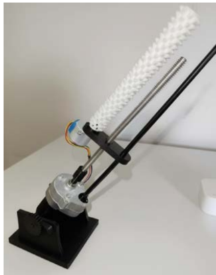
Figure 4. Conditioned prototype for the tower with the components printed, which include the rigid coupling, the tower base and the inclined base.
