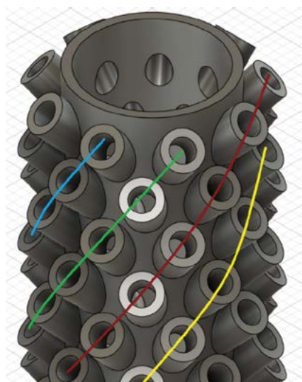
Figure 6. Movement projection of the greenhouse tower. The colored lines indicate its trajectory, which follows a spiral path.
