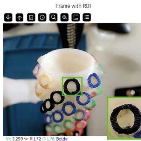
Figure 10. ROI creation within the frame: 2 windows were programmed in which the main window shows the complete frame and the ROI in green, the small window is a frame where only what the ROI detects is shown.
