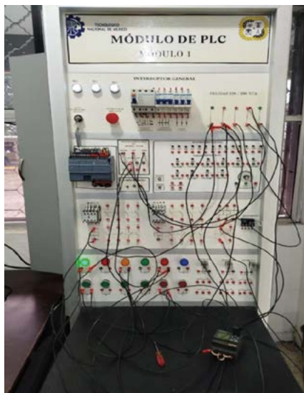
Figure 4. Physical wiring of the system in the PLC test module.
