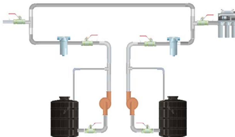
Figure 2. Diagram of the pumping and filtration system in the vanilla extract ingredient mixing process.
