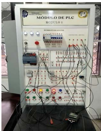
Figure 5. Practical demonstration of failure/precaution: activation of shutdown and failure/precaution indicators.
