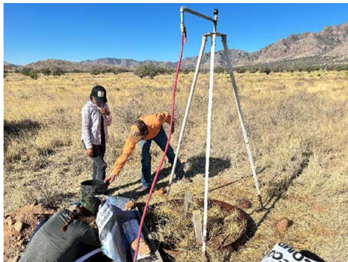
Figure 3. Rainfall simulator used to determine runoff, infiltration, and sediment yield.
