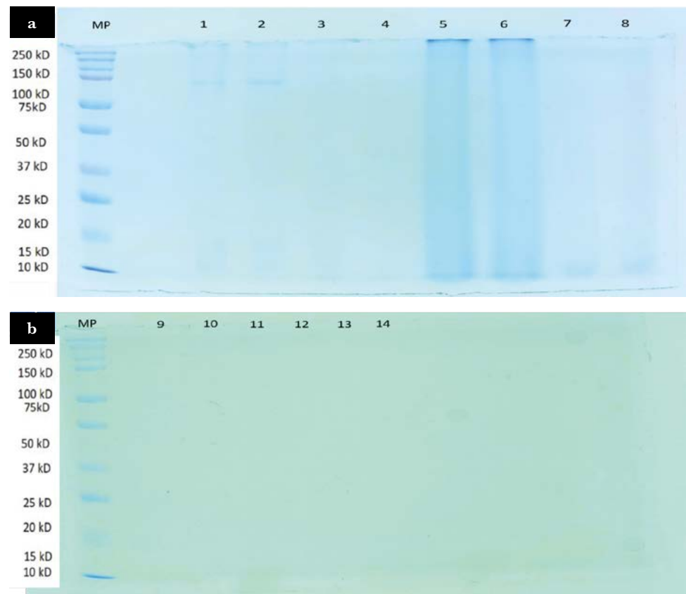
Figure 1. SDS-PAGE of the different hydrolyzed feather treatments. 1a: Lane MP: Standard protein marker; Lane 1 and 2: whole feathers; Lane 3 and 4: thermal hydrolysates; Lane 5 and 6: chemical hydrolysates; Lane 7 and 8: alkaline enzymatic hydrolysates. 1b: Lane MP: Standard protein marker; Lane 9 and 10: acidic enzymatic hydrolysates; Lane 11 and 12: liquid alkaline enzymatic hydrolysates; Lane 13 and 14: liquid acidic enzymatic hydrolysates.
