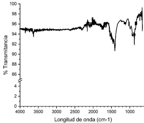
**Figure 6.** Spectrum of calcined oyster shell sample.
