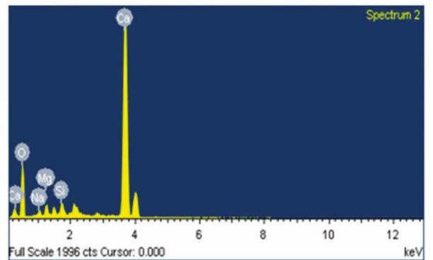
**Figure 4.** Elemental composition of calcined oyster shells.
